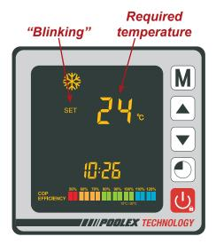
Once the symbol stops blinking, the required temperature is validated and is replaced by the water's current temperature (27° in our example).
