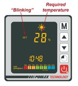
Once the symbol stops blinking, the required temperature is validated and is replaced by the water's current temperature (25° in our example).
