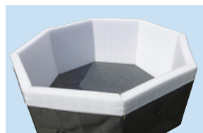
Insulating foam structure (13 cm thickness)
